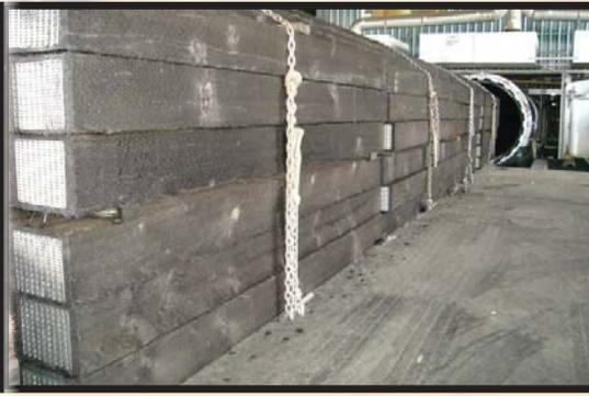
**CONDUCTIVITY.** Tests have indicated that the metallic oxides in ACZA are not conductive. Regardless of the test method used, a bigger factor than wood species or preservative was moisture, which affects all types of treated wood cross-ties.
